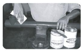
6 Wipe off excess solvent cement from the joint.
