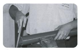
Remove internal and external burr and clean out swart.
